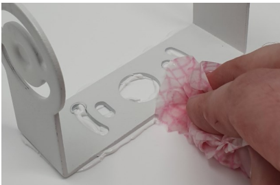
Wipe excess sealant away
